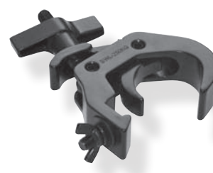
#8016-B Quick Selflock Coupler Black, 250kg (551lbs), 48-51mm (1.9-2.0") FT31-TT74
