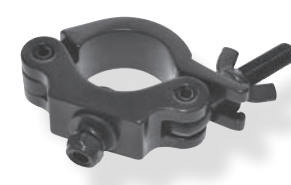
#8002-B Halfcoupler M10 Black, 200kg (440lbs), 48-51mm (1.9-2.0") FT31-TT74
