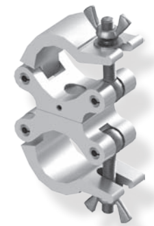
#8003 Swivel Coupler, 500kg (1100lbs), 48-51mm (1.9-2.0"), FT31-TT74
