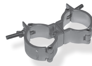
#8015 Swivel Coupler Slim, 100kg (220lbs), 48-51mm (1.9-2.0"), FT31-TT74
