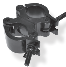
#8003-B Swivel Coupler Black, 500kg (1100lbs), 48-51mm (1.9-2.0") FT31-TT74
