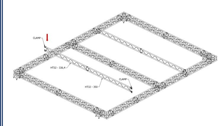
The exact position of the HT32-336,4 will be defined in the next step using inclined tubes.
