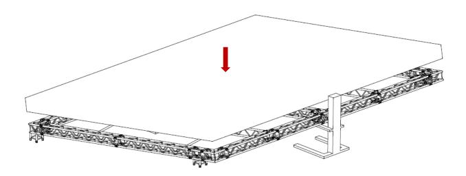
Before starting to lift the structure, fix cross bracing on three sides with cables and ropes.
